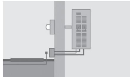
The GenReady load center is installed with the EZ Transfer operator. All fuel and electrical lines (contractor supplied) are installed to the planned generator site along with the generator pad (if required). The home is completely wired and ready for the addition of a generator in the future.
