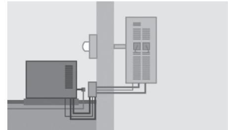
Everything included in the GenReady Advanced level is installed along with an automatic standby generator. The home's selected circuits will be backed up by generator power whenever the utility is lost.
