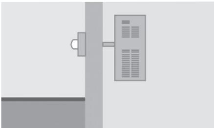
The GenReady load center is installed without the EZ Transfer operator. It replaces the home's main load center. This option will save the homeowner thousands in upgrade costs when a generator is installed.
